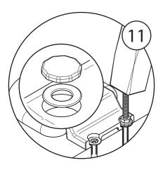
Place a washer and then a hammer-in plug in each hole. Use the M8 bolt again to hammer the plugs in firmly.
