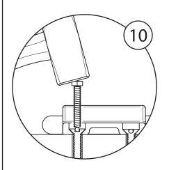
Place ball bearings in the boltheads. Using the smaller M8 bolt as a punch, hammer the bearings in.
