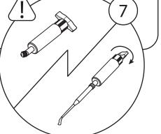
Remove the cap from the resin cartridge and screw on the mixer nozzle. On an unimportant surface, twist the plunger until a consistent grey resin ejects.
