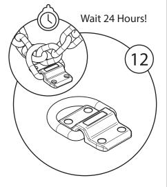
The Torc Ground Anchor is now installed. Please leave 24 hours before disturbing it or using it so the resin can set fully.
