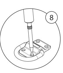
Through the baseplate AND FITTED D-SHACKLE, fill approximately 2/3rds of a hole with the resin.
