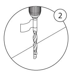
Drill the hole perpendicular to the surface about half way to the tape. Do not drill to the tape yet. If it is difficult to keep the drill positioned, drill an 8mm pilot hole first.
