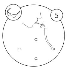
Use the tube to blow dust from the holes and use the test tube brush and a vacuum cleaner to clear remaining dust. HOLES MUST BE FREE OF DUST.
