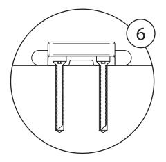
Place the product over the drilled, cleaned holes, and insert the bolts to check the holes are deep enough.
