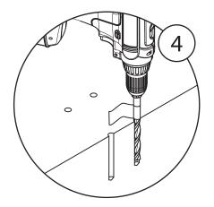
Move the anchor and drill the holes until the tape touches the mounting surface (95mm depth). Do not drill too deep.
