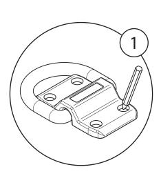
Place the anchor at an appropriate location (see page 1), check the D-Shackle fits, and mark a drilling hole.
