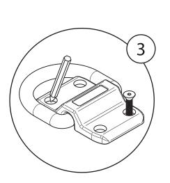
Place a bolt in the drilled hole for stability and mark the diagonally opposite hole. Repeat steps 1 - 3 until all holes are part drilled.
